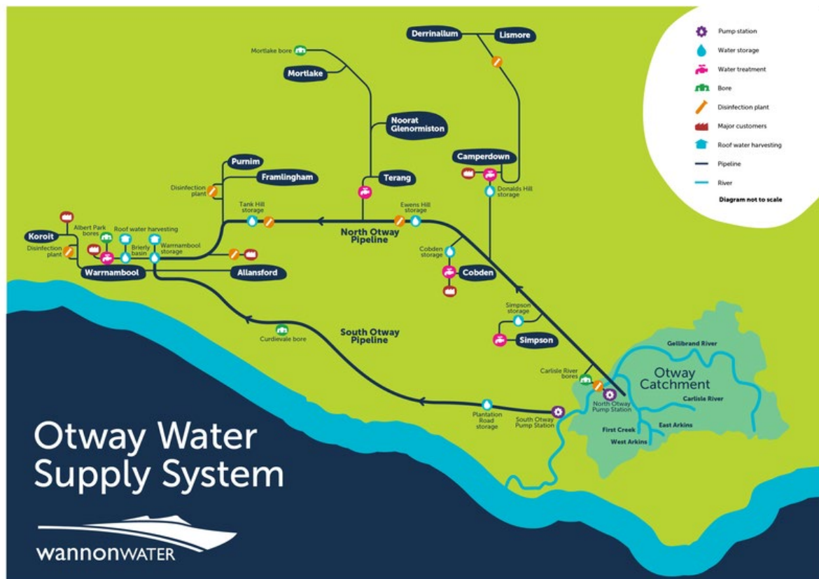
Figure 6 - Otways System Supply Schematic
